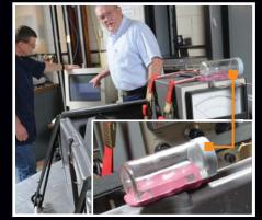
The water in the jar demonstrate to engineers the intense vibration a case withstands, while the jar attached to the equipment is calm, indicating a safe shock level (Shock mount technology does not apply to ProRack Cases).
