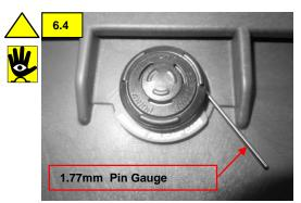
Note: Do not use any type of hammer in installing the PRV assembly.
