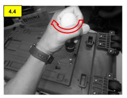
Note: If using a power tool, make sure to calibrate the tool first to 15.0 kg-cm torque to avoid stripping the screws due to over torqueing.
